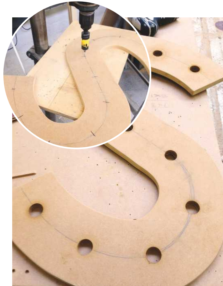
▲ Pic.6 The lampholders which I bought required a 30mm mounting hole. I didn't have a drill bit this size, so I had to use a holesaw. As I was using a holesaw, I thought it best to use my pillar drill. Not only does using a pillar drill make sure all the holes are straight, but it is much safer – I knew a guy who had his wrist snapped by a holesaw that got stuck, so drill, drill, drill! It was only once I had drilled all of my holes that I noticed my mistake from earlier – one too many holes! Damn it! So I needed to get another light bulb and holder, which was a tad annoying! Make sure you check your work before cutting!
